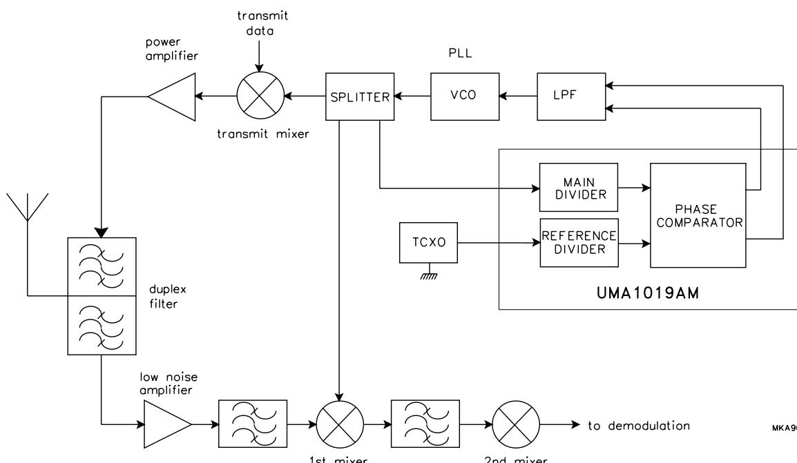
Fig.4 Typical application block diagram.
