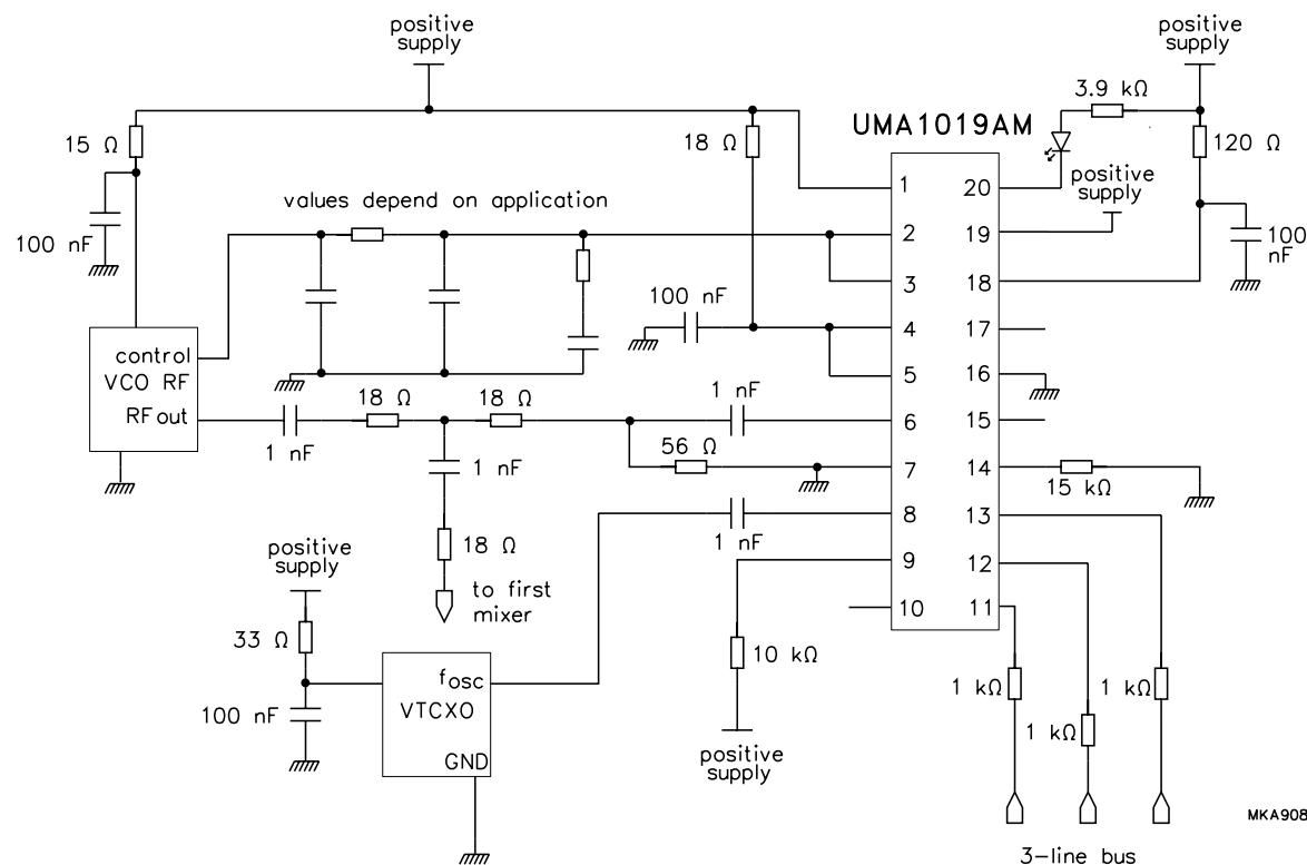
Fig.5 Typical test and application diagram.
