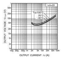
Fig.4 Output voltage vs. output current
