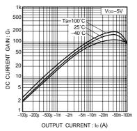
Fig.7 DC current gain vs. output
