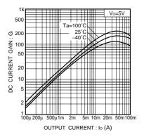
Fig.3 DC current gain vs. output
