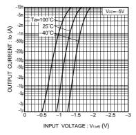
Fig.6 Output current vs. input voltage (OFF characteristics)
