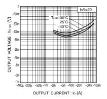
Fig.8 Output voltage vs. output current
