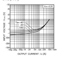
Fig.5 Input voltage vs. output current (ON characteristics)
