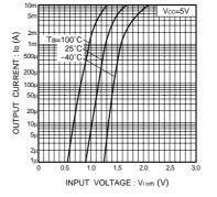
Fig.2 Output current vs. input voltage (OFF characteristics)
