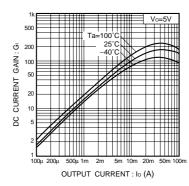
Fig.3 DC current gain vs. output current
