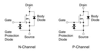
**Remark** The diode connected between the gate and source of the transistor serves as a protector against ESD. When this device actually used, an additional protection circuit is externally required if a voltage exceeding the rated voltage may be applied to this device.
