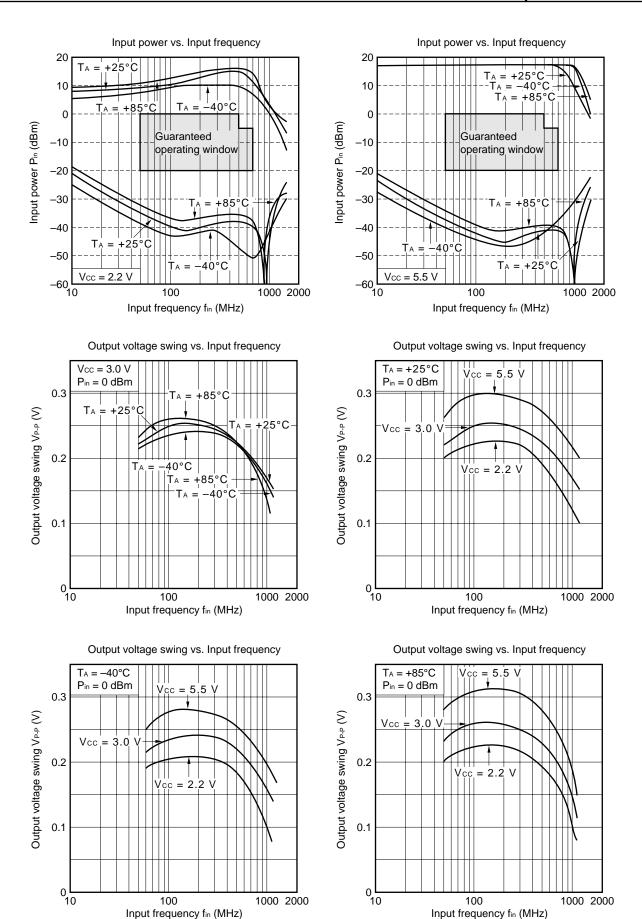
Divide by 4 mode (Guaranteed operating window: Vcc = 2.2 to 5.5 V,  $T_A = -40$  to +85°C)
