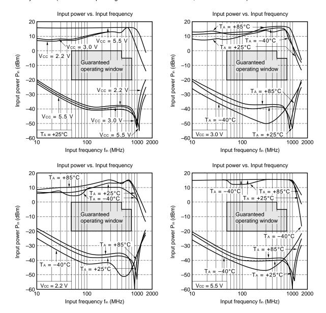
Divide by 8 mode (Guaranteed operating window: Vcc = 2.2 to 5.5 V,  $T_A = -40$  to +85°C)
