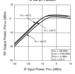
RF OUTPUT POWER vs. IF INPUT POWER
