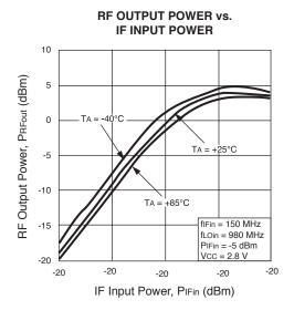
RF OUTPUT POWER vs. IF INPUT POWER
