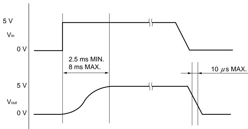
The above figure does not show the actual waveform. For the related characteristic waveform, refer to Major Characteristic Curves.
