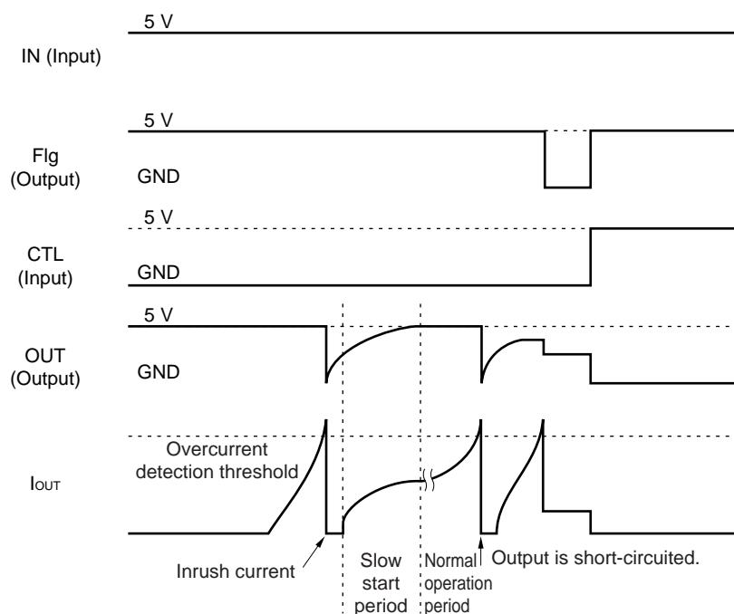
If an overcurrent is detected after the overcurrent detection delay time of  $20 \mu\text{s}$ , the IC executes a slow-start operation (output rise time:  $5 \text{ ms TYP.}$ ) again.
