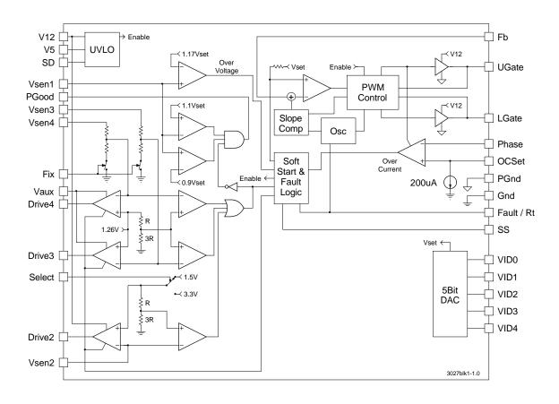
Figure 1 - Simplified block diagram of the US3027.
