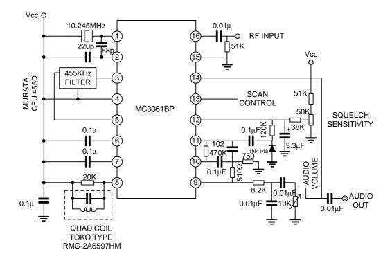
In the above typical application, the audio signal is recovered using a conventional quadrature FM detector. The absence of an input signal is indicated by the presence of noise above the desired audio frequencies. This "noise band: is monitored by an active filter and a detector. A squelch trigger circuit indicates the presence of noise (or a tone) by an output which can be used to control scanning. At the same time, an internal switch is operated which can be used to mute the audio.
