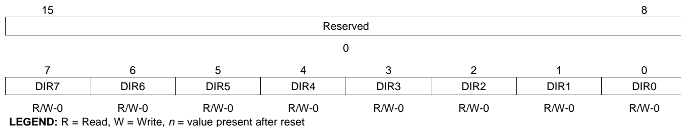
Figure 3-20. General-Purpose I/O Control Register (GPIOCR) [MMR Address 003Ch]
