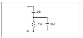
FIGURE 11. VCA2613 Input Impedance.
