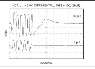
FIGURE 16. Overload Recovery Response For Maximum Gain.
