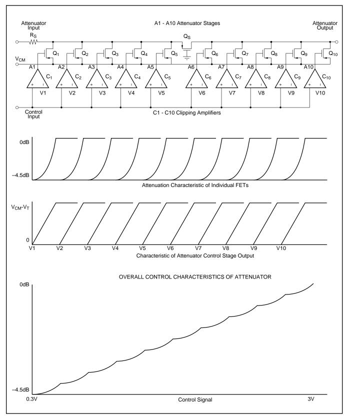
FIGURE 12. Piecewise Approximation to Logarithmic Control Characteristics.
