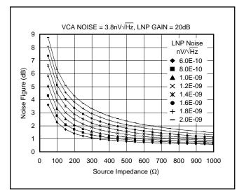
FIGURE 6. Noise Figure for Active Termination.
