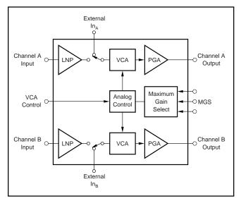
FIGURE 1. Simplified Block Diagram of the VCA2613.
