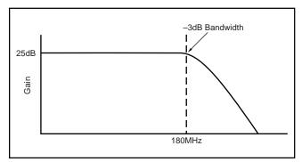
FIGURE 9. Open-Loop Gain Characteristic of LNP.
