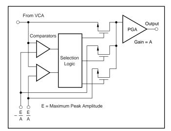
FIGURE 14. Overload Protection Circuitry.
