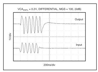
FIGURE 15. Overload Recovery Response For Minimum Gain.
