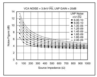
FIGURE 7. Noise Figure for Conventional Termination.
