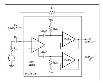
FIGURE 8. Low Frequency LNP Time Constants.
