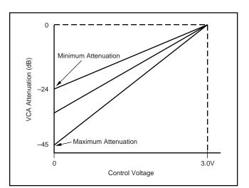
FIGURE 3. Swept Attenuator Characteristic.
