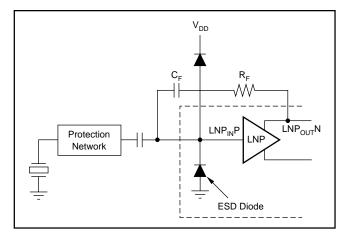
FIGURE 17. VCA2613 Diode Bridge Protection Circuit.
