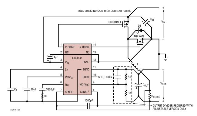
Figure 9. LTC1148 Layout Diagram (See Board Layout Checklist)
