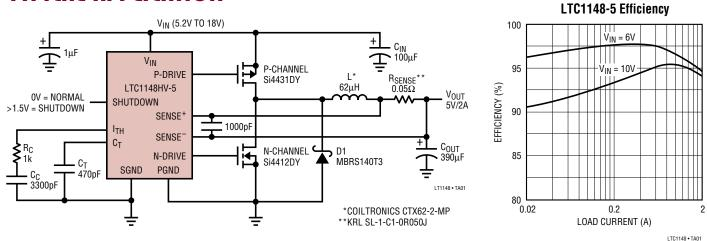
Figure 1. High Efficiency Step-Down Converter
