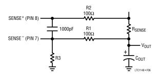
Figure 6. Suppression of Burst Mode Operation
