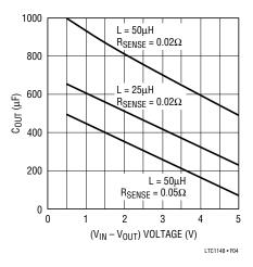
Figure 4. Minimum Value of  $\mathbf{C}_{\text{OUT}}$
