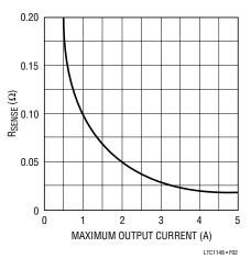
Figure 2. Selecting  $R_{\mbox{SENSE}}$
