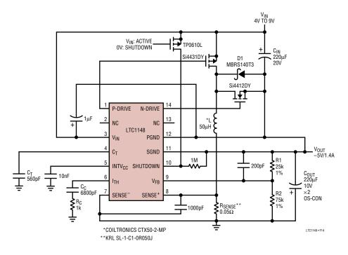
Figure 14. 4V to 9V Input Voltage to -5V/1A Regulator
