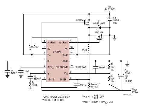
Figure 12. High Efficiency Adjustable 3A Regulator
