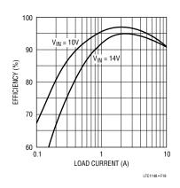
Figure 19. All N-Channel 5V/8A Efficiency
