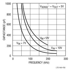
Figure 3. Timing Capacitor Value
