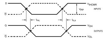
FIGURE 1. Differential to Differential Propagation Delay
