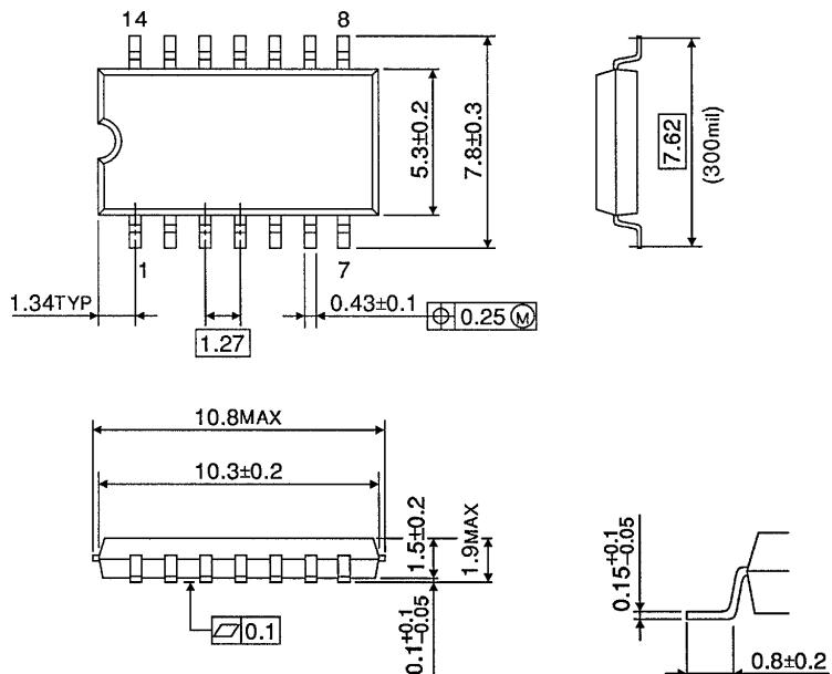
**SOP 14PIN (150mil BODY) PACKAGE DIMENSIONS (SOL14-P-150-1.27)**
