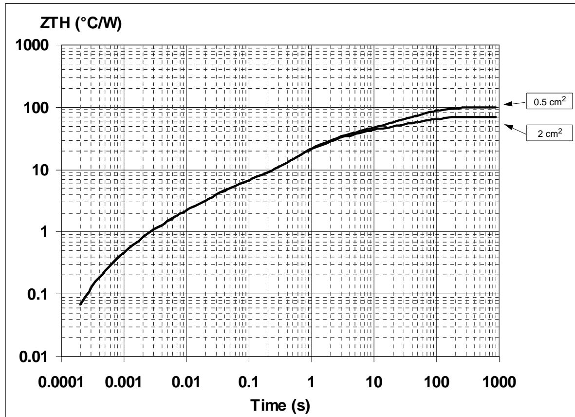
**Thermal fitting model of a single channel HSD in SO-8**
