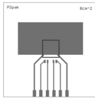
Layout condition of  $R_{th}$  and  $Z_{th}$  measurements (PCB FR4 area= 60mm x 60mm, PCB thickness=2mm, Cu thickness=35μm, Copper areas: 0.97cm<sup>2</sup>, 8cm<sup>2</sup>).
