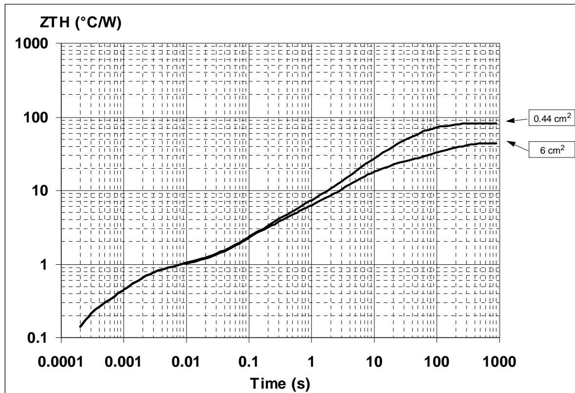
**Thermal fitting model of a single channel HSD in PPAK**
