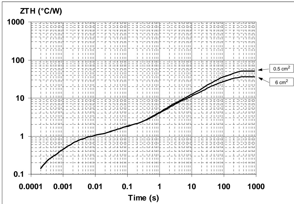
Thermal fitting model of a single channel HSD in P<sup>2</sup>PAK
