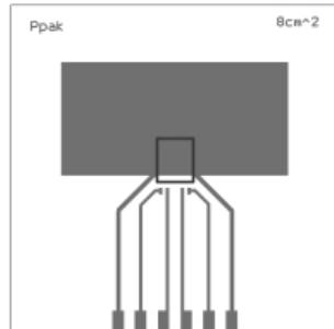
Layout condition of  $R_{th}$  and  $Z_{th}$  measurements (PCB FR4 area= 60mm x 60mm, PCB thickness=2mm, Cu thickness=35 $\mu$ m, Copper areas: 0.44cm $^2$ , 8cm $^2$ ).
