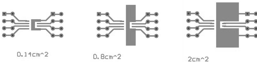
Layout condition of  $R_{th}$  and  $Z_{th}$  measurements (PCB FR4 area= 58mm x 58mm, PCB thickness=2mm, Cu thickness=35μm, Copper areas: 0.14cm<sup>2</sup>, 0.8cm<sup>2</sup>, 2cm<sup>2</sup>).
