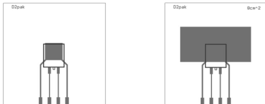
Layout condition of  $R_{th}$  and  $Z_{th}$  measurements (PCB FR4 area= 60mm x 60mm, PCB thickness=2mm, Cu thickness=35µm, Copper areas: from minimum pad lay-out to 8cm<sup>2</sup>).
