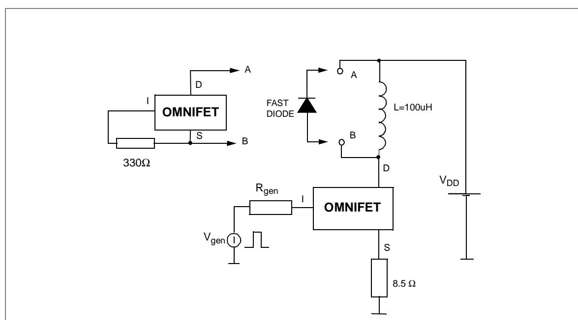
**Figure 3:** Unclamped Inductive Load Test Circuits
