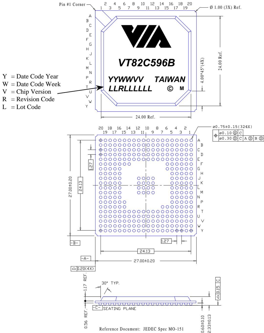
**Figure 16. Mechanical Specifications - 324-Pin Ball Grid Array Package**
