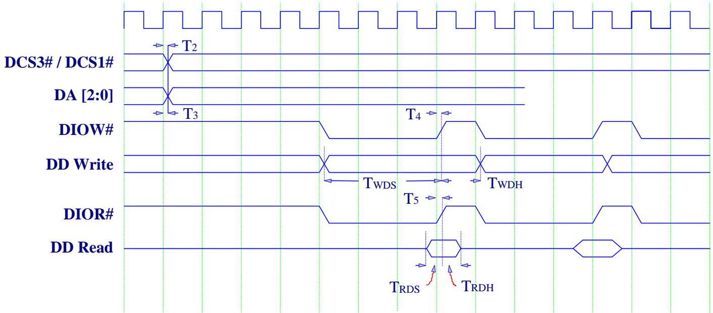
Figure 15. UltraDMA-33 IDE Timing - PIO Cycle
