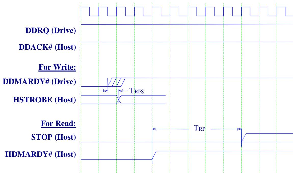
**Figure 10. UltraDMA-33 IDE Timing - Pausing a DMA Burst**
