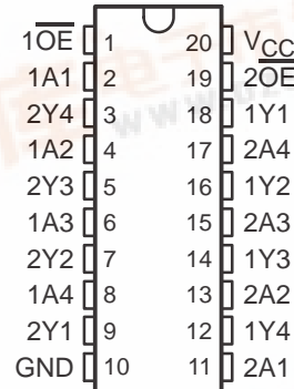
SN54LVTZ244 ... J PACKAGE SN74LVTZ244 ... DB, DW, OR PW PACKAGE (TOP VIEW)
