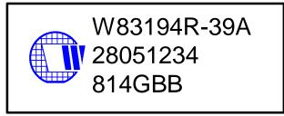
1st line: Winbond logo and the type number: W83194R-39/-39A 2nd line: Tracking code <u>2</u> 8051234 <u>2</u>: wafers manufactured in Winbond FAB 2 <u>8051234</u>: wafer production series lot number 3rd line: Tracking code <u>814 G B B</u> <u>814</u>: packages made in '<u>98</u>, week <u>14</u> <u>G</u>: assembly house ID; A means ASE, S means SPIL, G means GR
