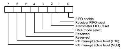
Notes: Bit 6, 7: These two bits are used to set the active level for the receiver FIFO interrupt. For example, if the interrupt active level is set as 4 bytes, once there are more than 4 data characters in the receiver FIFO, the interrupt will be activated to notify the CPU to read the data from the FIFO.
