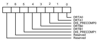
This register controls the data rate selection for FDC. It also controls if precompensation is enabled. DRTA1, DRTA0 (bit 1 - bit 0):
