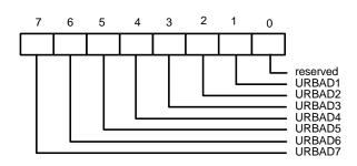
This register is used to select the base address of the UART B from 100H-3F8H on 8-byte boundaries. NCS = 0 and A10 = 0 are required to access the UART B registers. A[2:0] are don't-care conditions.
