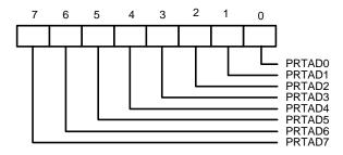
This register is used to select the base address of the parallel port. If EPP is disable, the parallel port can be set from 100H-3FCH on 4-byte boundaries. If EPP is enable, the parallel port can be set from 100H-3F8H on 8-byte boundaries. NCS = 0 and A10 = 0 are required to access the parallel port when in compatible, bi-directional, or EPP modes. A10 is active in ECP mode.
