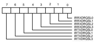
IRTXDRQSL (bit 7-bit 4): Transmitter DMA channel A through D selection when high speed infrared (FIR/MIR) is used and enable DMA channel. Note that these bits is used in two DMA channels.
