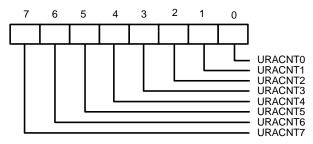
URACNT7 - URACNT0 (Bit 7 - bit 0): UART A idle timer count.
