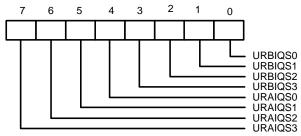
URAIQS3-URAIQS0 (Bit 7-bit 4): Allocate interrupt resource for UART A. URBIQS3-URBIQS0 (Bit 3-bit 0): Allocate interrupt resource for UART B.
