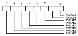
PM1AD7 - PM1AD2 (Bit 7 - bit 2): Base address of the power management register block PM1.
