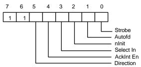
Bit 6, 7: These two bits are logic one during a read and cannot be written.
