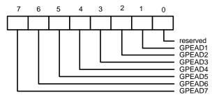
GPEAD7 - GPEAD1 (Bit7 - bit 1): Base address of the power management register block GPE.
