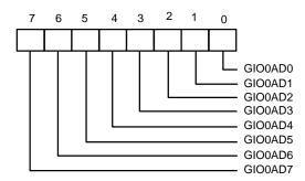
GIO0AD7-GIO0AD0 (Bit 7-bit 0): GIOP0 (pin 92) address bit 7 - bit 0.
