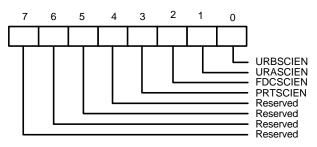
These bits are used to enable the device's IRQ sources onto the SCI logic. The SCI logic output for the IRQs is as follows:
