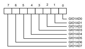
GIO1AD7-GIO1AD0 (Bit 7-bit 0): GIOP1 (pin 96) address bit 7-bit 0.
