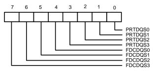
FDCDQS3-FDCDQS0 (Bit 7-bit 4): Allocate DMA resource for FDC.
