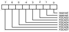
This register is used to select the base address of the Floppy Disk Controller (FDC) from 100H-3F0H on 16-byte boundaries. NCS = 0 and A10 = 0 are required to access the FDC registers. A[3:0] are always decoded as 0xxxb.
