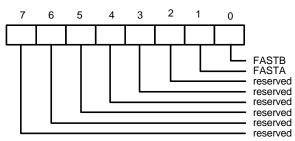
This register is used for the high speed modem application. While the bit is set to logic 1, it can increase the baudrate of UART to 921.2KBPS (the clock source of UART is 14.769MHz) for high speed transmit/receive.
