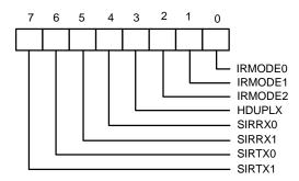
SIRTX1 (Bit 7): IRTX pin selection bit 1
