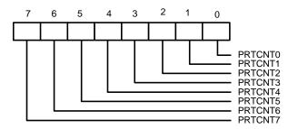
PRTCNT7 - PRTCNT0 (Bit 7 - bit 0): printer port idle timer count.
