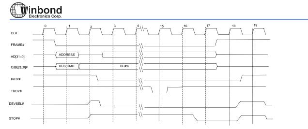
Because W89C940 don't support memory command in burst mode. When the host try to send memory command in burst mode, the first data phase is completed. TRDY# and IRDY# are deasserted, but the FRAME# is asserted for the next data phase. The device will assert STOP# to terminate the transaction. Data is not transferred after STOP# is asserted. The host need to initiate another transaction for further data transfer. The timing is shown above.
