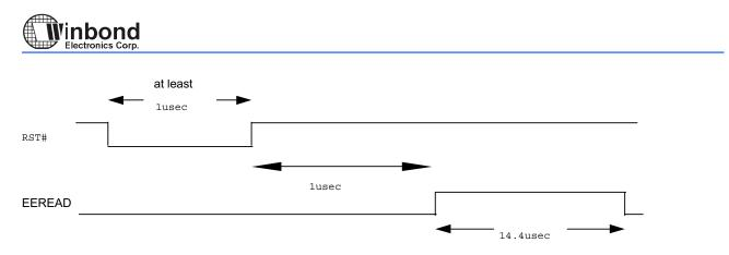
Since the ELANC-PCI reloads data into the configuration registers each time the system is reset, caution should be taken in handling resets. A system reset should keep low at least 480ns for the ELANC-PCI to decode the action as a reset. Any signal on the RESET pin shorter than this will be interpreted as noise and no response will be taken by the ELANC-PCI.
