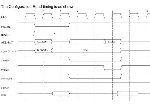
The timing is the same as the figure I/O Read Transaction, except the IDSEL is asserted during the address phase. The transaction access the configuration registers of the device.
