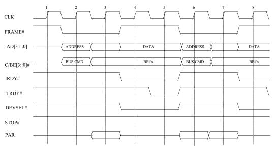
Without contention of TRDY#, DEVSEL#, or STOP#, the IDLE states between transactions are removed. It increase the throughput of the data transaction. If the first transaction is a write cycle and the second transaction access( can be read or write transaction) to the same target , one IDLE cycle can be removed between transactions.
