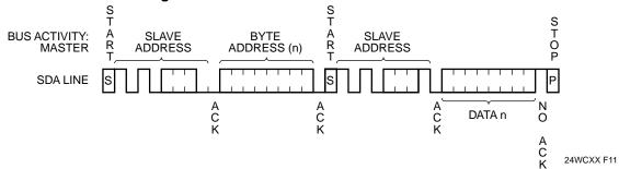
Figure 10. Sequential Read Timing
