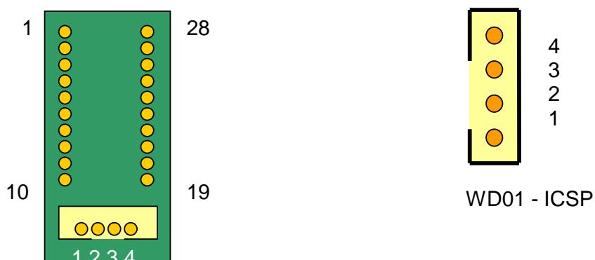
Adaptor plugs into top of ZIF socket on programmer. Cable is pin-to-pin
