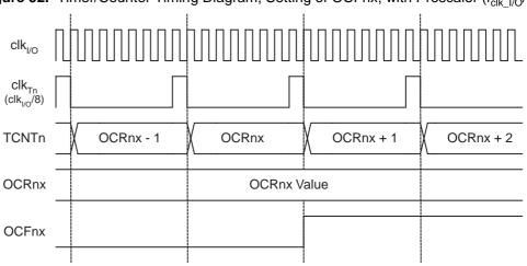
Figure 52. Timer/Counter Timing Diagram, Setting of OCFnx, with Prescaler (f<sub>clk I/O</sub>/8)
