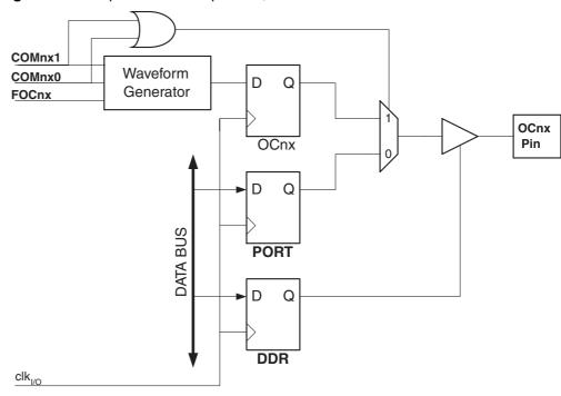
Figure 46. Compare Match Output Unit, Schematic
