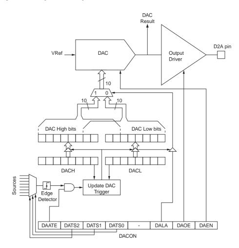
Figure 131. Digital to Analog Converter Block Schematic
