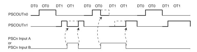
Figure 81. PSC behaviour versus PSCn Input A or Input B in Fault Mode 4
