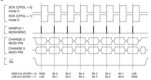
Figure 97. SPI Transfer Format with CPHA = 1
