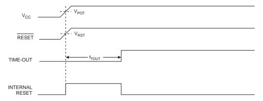
Figure 19. MCU Start-up, RESET Extended Externally
