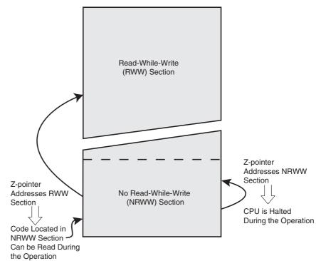
Figure 133. Read-While-Write vs. No Read-While-Write
