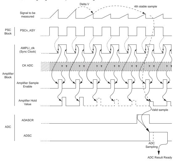
Figure 129. Amplifier synchronization timing diagram
