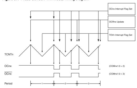
Figure 37. Phase Correct PWM Mode, Timing Diagram
