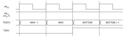
Figure 39 shows the same timing data, but with the prescaler enabled.
