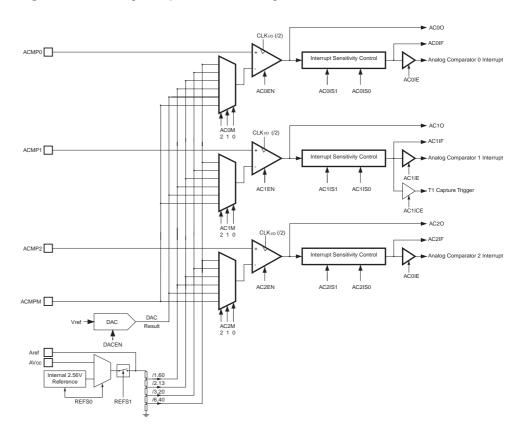
Figure 114. Analog Comparator Block Diagram<sup>(1)(2)</sup>
