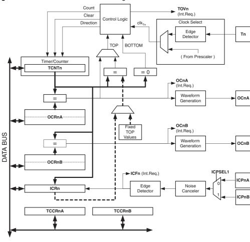
Figure 42. 16-bit Timer/Counter Block Diagram<sup>(1)</sup>
