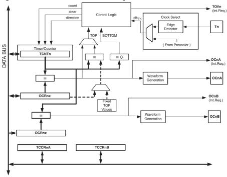
Figure 31. 8-bit Timer/Counter Block Diagram
