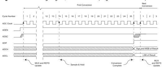
Figure 118. ADC Timing Diagram, First Conversion (Single Conversion Mode)
