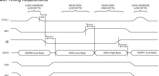
$\textbf{Figure 144.} \ \, \text{Parallel Programming Timing, Reading Sequence (within the Same Page)} \\ \, \text{with Timing Requirements}^{(1)}$
