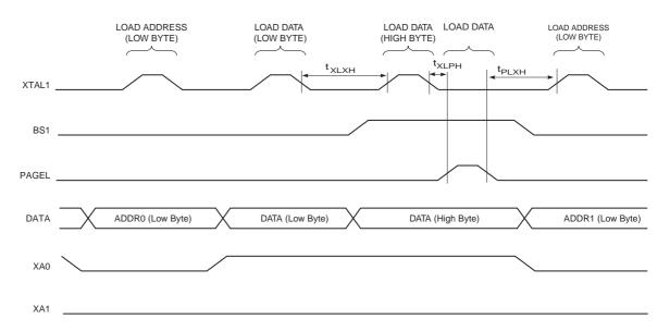
Note: 1. The timing requirements shown in Figure 151 (i.e., t<sub>DVXH</sub>, t<sub>XHXL</sub>, and t<sub>XLDX</sub>) also apply to loading operation.
