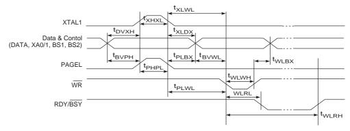
**Figure 143.** Parallel Programming Timing, Loading Sequence with Timing Requirements<sup>(1)</sup>
