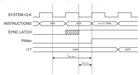
Figure 26. Synchronization when Reading an Externally Applied Pin value
