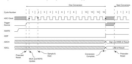
Figure 121. ADC Timing Diagram, Free Running Conversion
