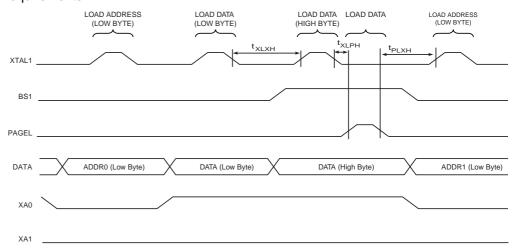
Note: 1. The timing requirements shown in Figure 142 (i.e., t<sub>DVXH</sub>, t<sub>XHXL</sub>, and t<sub>XLDX</sub>) also apply to loading operation.
