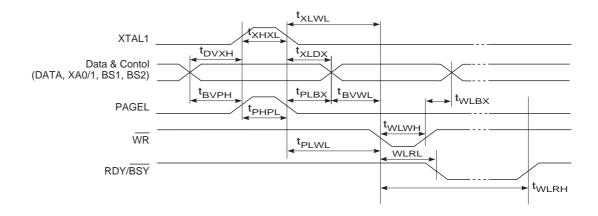
**Figure 152.** Parallel Programming Timing, Loading Sequence with Timing Requirements<sup>(1)</sup>
