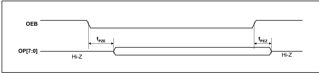
Figure 3 Output Data Enable Timing
