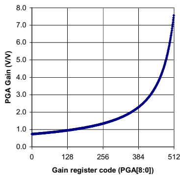
Figure 9 Wide Range Gain Mode (PGAMODE=0) Figure 10 High-Res Gain Mode (PGAMODE=1)
