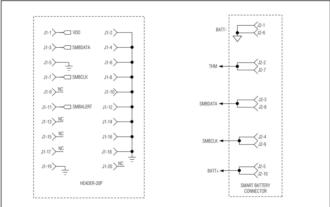
Figure 5. MAX1535B EV Kit Schematic—Smart Battery Connector
