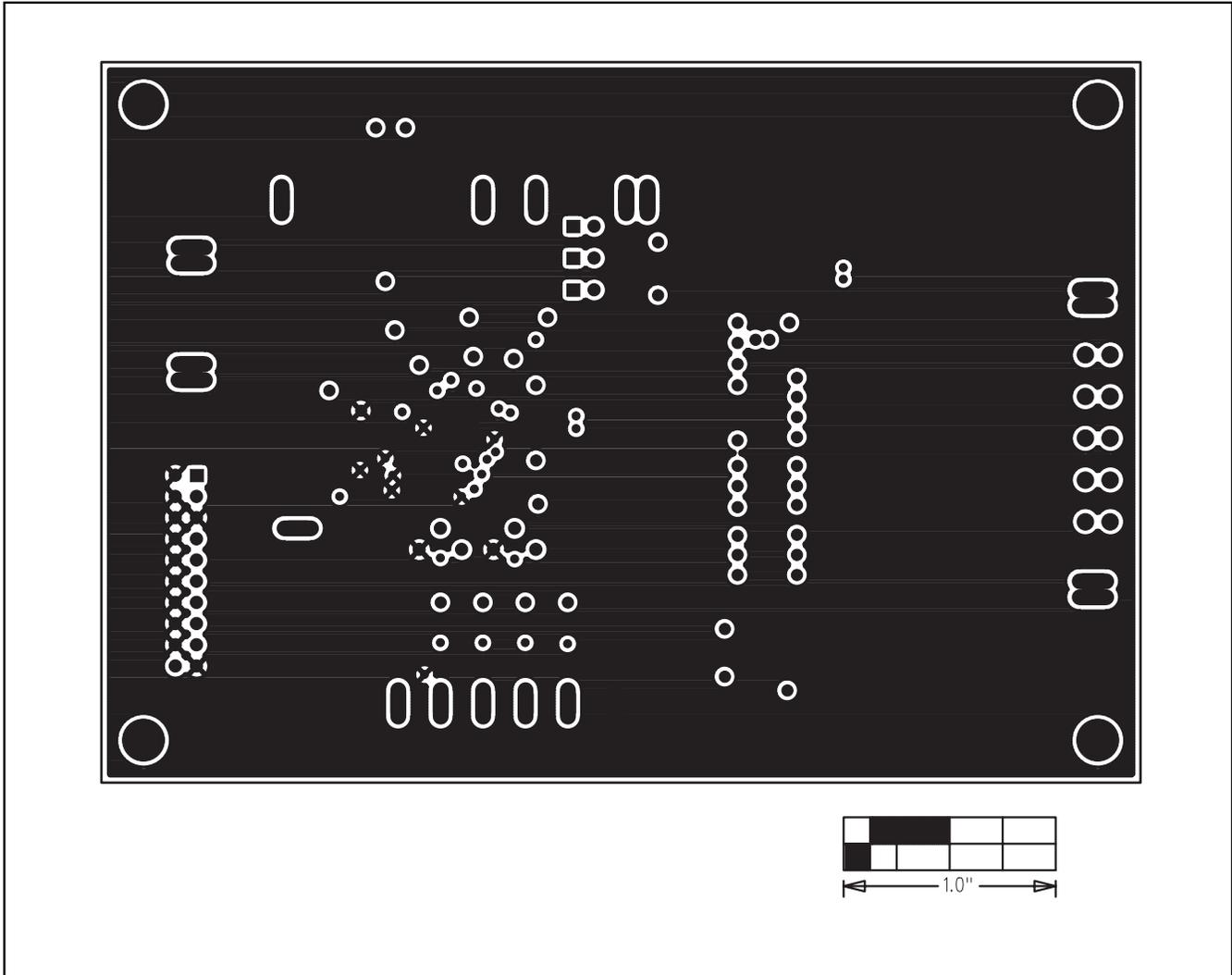
Figure 9. MAX1535B EV Kit PC Board Layout—Ground Plane
