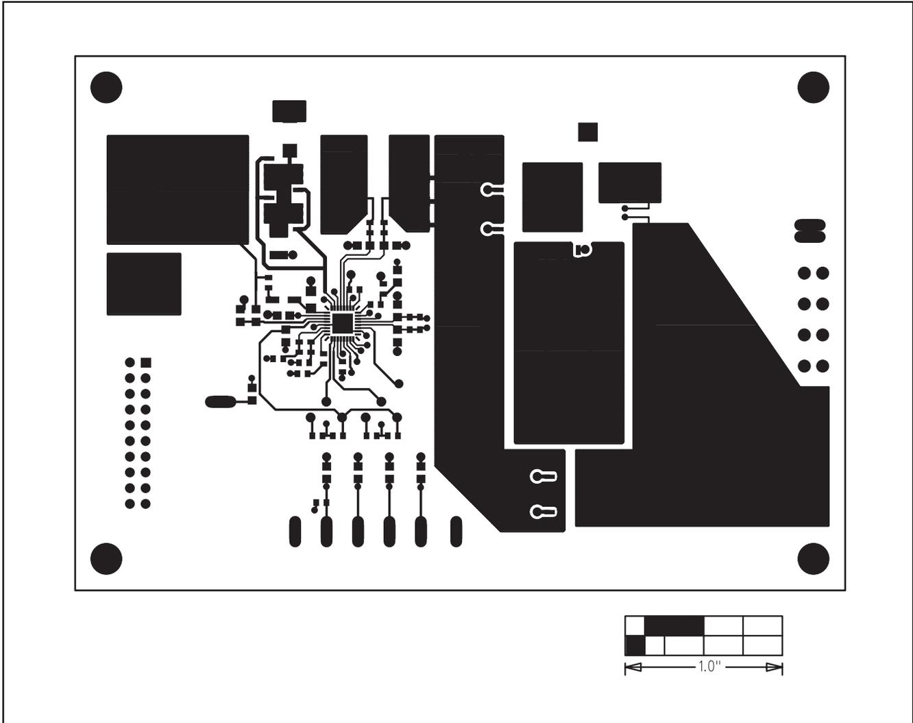
Figure 7. MAX1535B EV Kit PC Board Layout—Component Side
