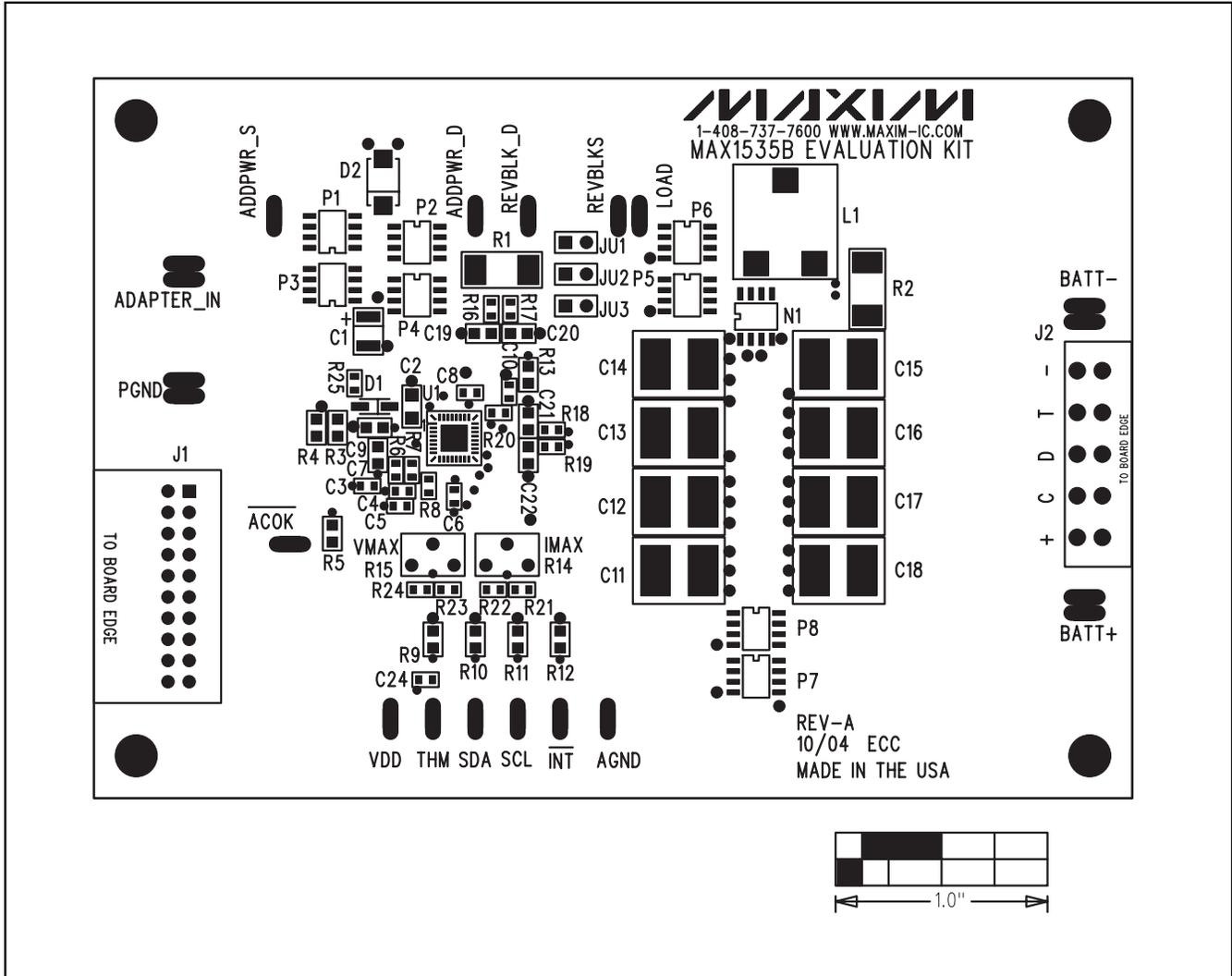
Figure 6. MAX1535B EV Kit Component Placement Guide—Component Side
