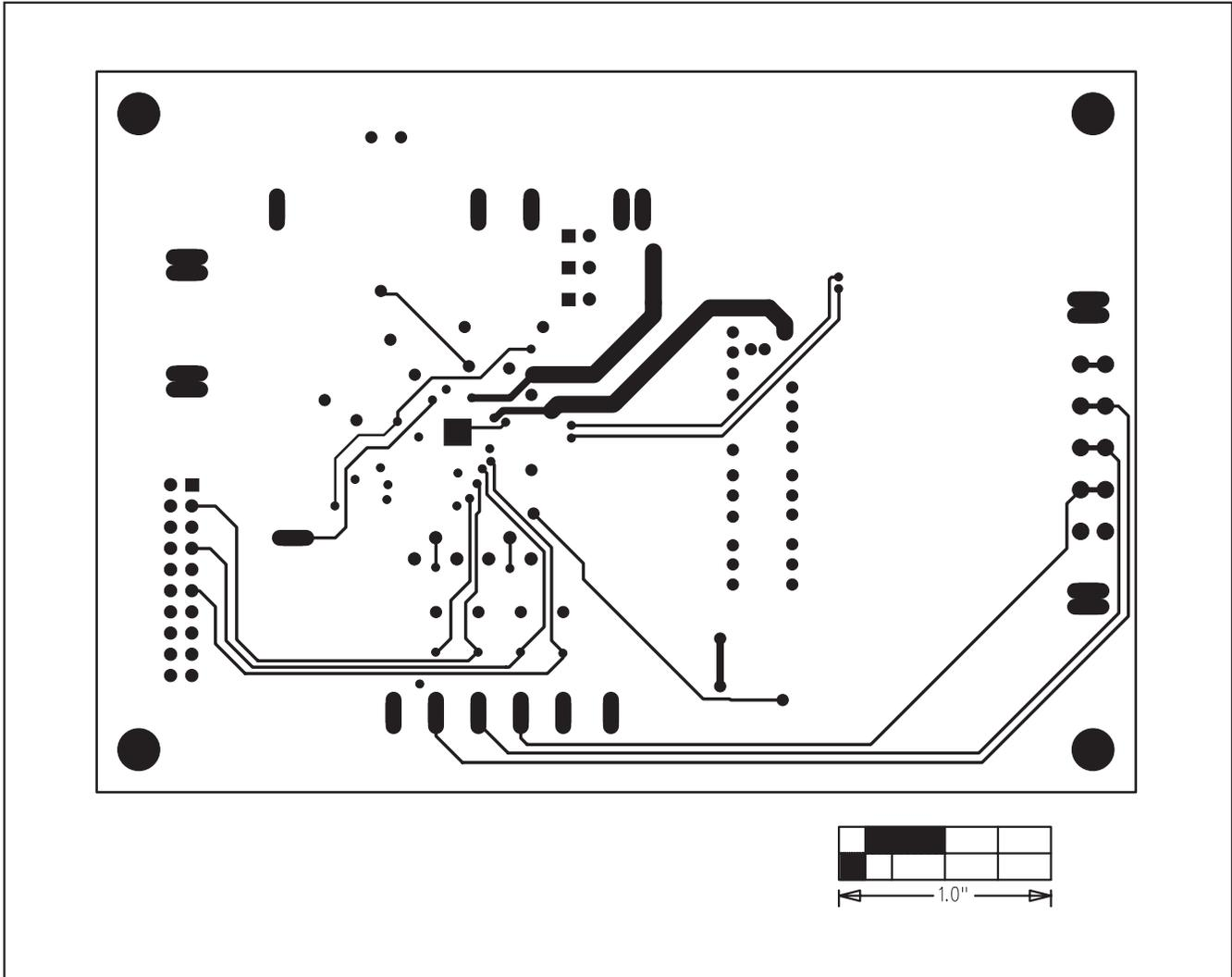
Figure 10. MAX1535B EV Kit PC Board Layout—Solder Side
