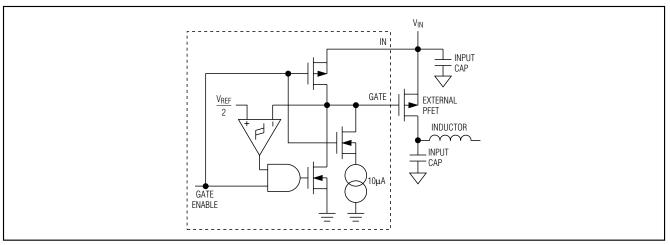
Figure 6. External P-Channel MOSFET Input Switch Control
