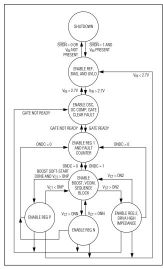
Figure 7. Power-Up Sequence State Diagram
