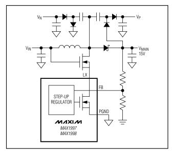
Figure 13. Operation with Output Voltage >13V Using Cascoded MOSFET
