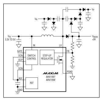
Figure 14. Disabling Input MOSFET Switch
