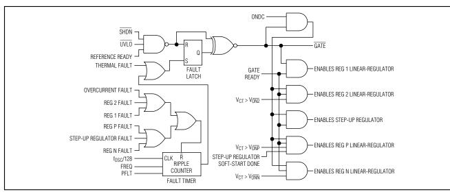
Figure 8. Startup and Fault Protection Logic
