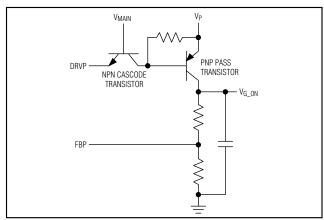
Figure 4. Using Cascode NPN for Output Voltages > 28V
