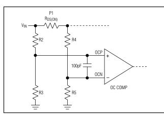
Figure 10. Setting the Overcurrent Threshold
