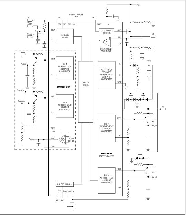
Figure 2. System Functional Diagram
