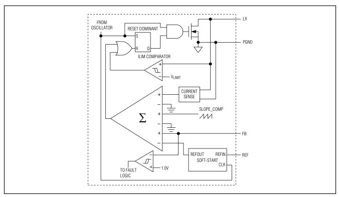
Figure 3. Main Step-Up Converter Functional Diagram
