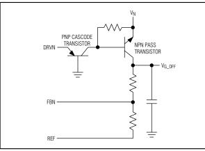
Figure 5. Using Cascode PNP for Output Voltages < VIN - 28V
