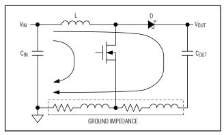
Figure 12. High-Current Loops of Step-Up Regulator
