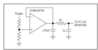
Figure 11. Optimizing VCOM Buffer Drive Current
