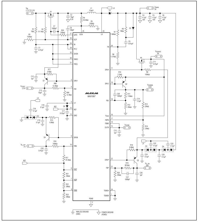
Figure 1. Standard Application Circuit
