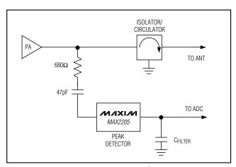
Figure 2. MAX2205 Typical Application Circuit
