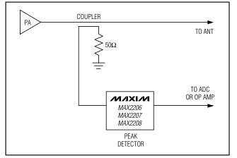
Figure 1. MAX2206/MAX2207/MAX2208 Typical Application Circuit
