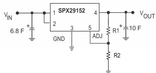
Figure 1. Fixed Output Linear Regulator
