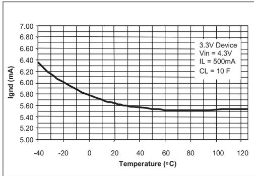
Figure 11. Ground Current vs Temperature at  $I_{LOAD}=500$
