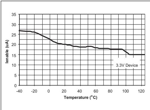
Figure 17. ENABLE Current vs Temperature at  $V_{EN} = 16V$
