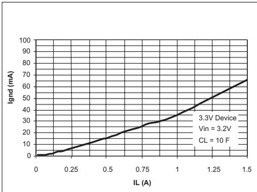
Figure 7. Ground Current vs Load Current in Dropout
