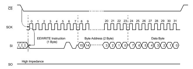
Figure 12. EEPROM Byte Write (EEWRITE) Operation Sequence
