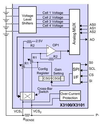
The internal gain of the X3100 or X3101 current sense voltage amplifier can be selected by using the WCNTR Instruction to set bits CSG1 and CSG0 in the control register (Table 14). The CSG1 and CSG0 bits select one of four input resistors to Op Amp OP1. The feedback resistors remain constant. This ratio of input to feedback resistors determines the gain. Putting external resistors in series with the inputs reduces the gain of the amplifier.
