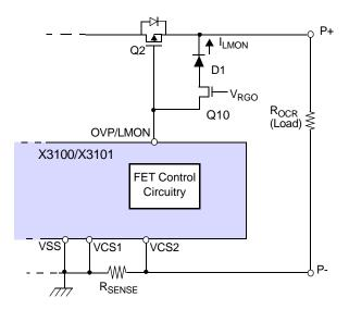
The 5VDC voltage regulator output ( $V_{RGO}$ ) is always active during an over-current protection mode.
