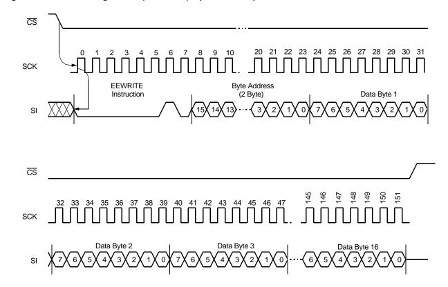
Figure 13. EEPROM Page Write (EEWRITE) Operation Sequence
