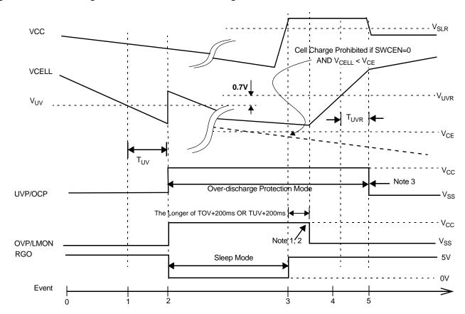
Figure 6. Over-discharge Protection Mode—Event Diagram
