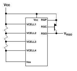
Increase Vcc until  $\rm V_{RGO}$  turns on
