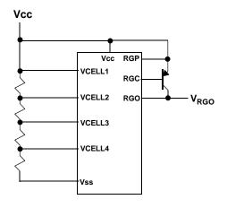
Increase Vcc until  $V_{RGO}$  turns on
