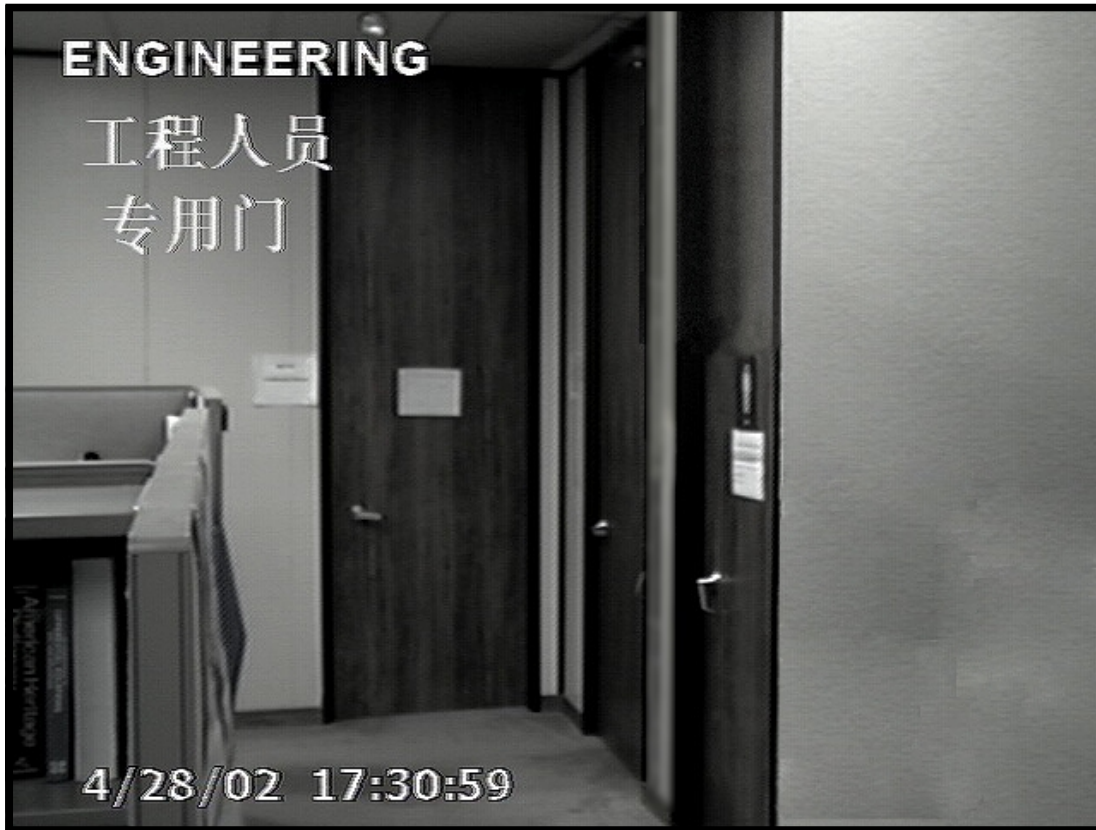
Figure 3. On-Screen Display Capability of the MAX4455
