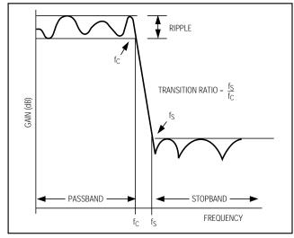
Figure 3. Elliptic Filter Response
