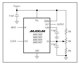
Figure 4. Offset Adjustment Circuit
