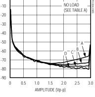
THD PLUS NOISE vs. INPUT SIGNAL **AMPLITUDE (MAX7407)**
