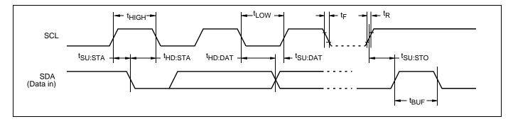
Figure 11. Output Bus Timing
