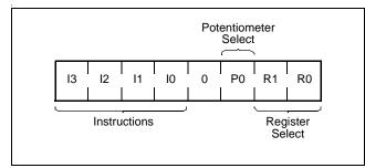
The four high order bits define the instruction. The sixth bit (P0) selects which one of the two potentiometers is to be affected by the instruction. The last two bits (R1 and R0) select one of the four registers that is to be acted upon when a register oriented instruction is issued.
