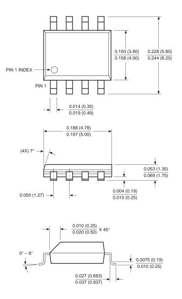
NOTE: ALL DIMENSIONS IN INCHES (IN PARENTHESIS IN MILLIMETERS)
