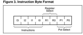
The four high order bits of the instruction byte specify the operation. The next two bits ( $R_1$  and  $R_0$ ) select one of the four registers that is to be acted upon when a register oriented instruction is issued. The last two bits ( $P_1$  and  $P_0$ ) selects which one of the four potentiometers is to be affected by the instruction.
