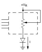
Two terminal Variable Resistor; Variable current
