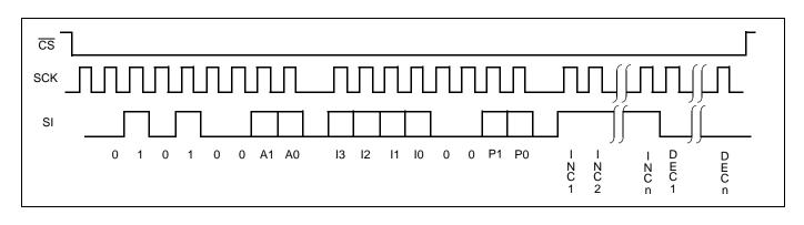
Figure 8. Increment/Decrement Timing Limits
