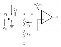
$\begin{array}{l} {Z_{IN}} = {R_2} + s\,{R_2}\left( {{R_1} + {R_3}} \right)C_1 = {R_2} + s\,\text{Leq} \\ ({R_1} + {R_3}) >> {R_2} \end{array}$
