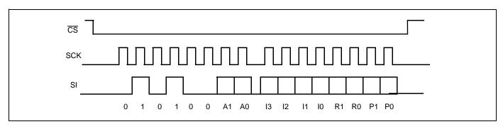
Figure 5. Three-Byte Instruction Sequence (Write)
