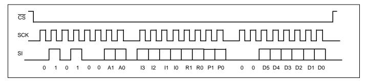
Figure 6. Three-Byte Instruction Sequence (Read)
