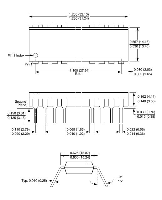
24-Lead Plastic Dual In-Line Package Type P
