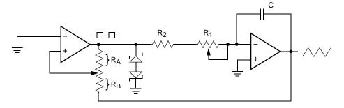
$\begin{array}{l} \mbox{frequency} \propto R_1,\,R_2,\,C \\ \mbox{amplitude} \propto R_A,\,R_B \end{array}$
