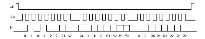
Figure 5. Three-Byte Command Sequence (Read)
