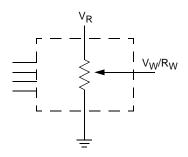
Three terminal Potentiometer; Variable voltage divider
