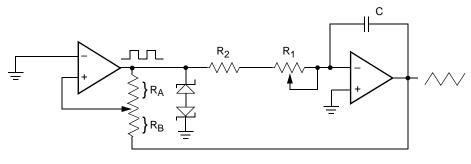
$\begin{array}{l} \text{frequency} \propto R_1,\,R_2,\,C \\ \text{amplitude} \propto R_A,\,R_B \end{array}$
