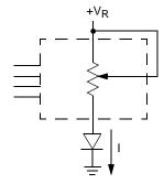
Two terminal Variable Resistor; Variable current
