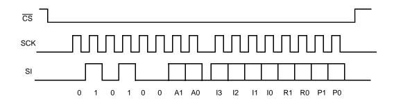
Figure 4. Three-Byte Command Sequence (Write)
