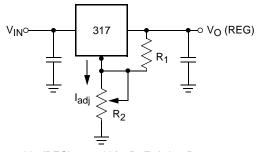
$V_{O}(REG) = 1.25V (1+R_2/R_1)+I_{adj} R_2$
