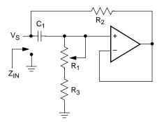
$$Z_{IN} = R_2 + s R_2 (R_1 + R_3) C_1 = R_2 + s \text{ Leq}$$
