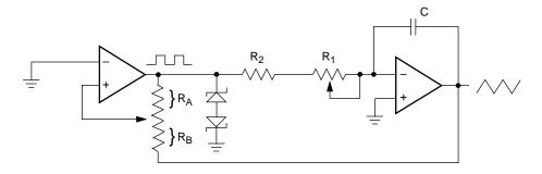
$\begin{array}{l} \text{frequency} \propto R_1,\,R_2,\,C \\ \text{amplitude} \approx R_A,\,R_B \end{array}$
