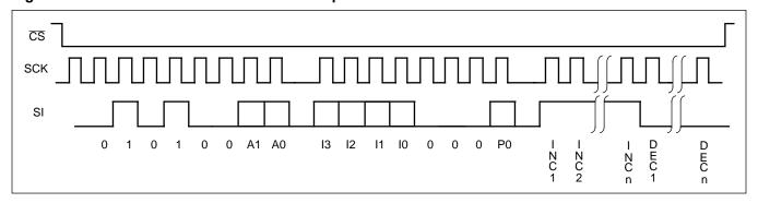
Figure 8. Increment/Decrement Timing Limits
