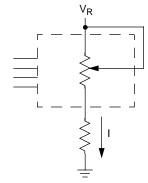
Two terminal Variable Resistor; Variable current
