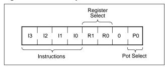
The four high order bits of the instruction byte specify the operation. The next two bits ( $R_1$  and  $R_0$ ) select one of the four registers that is to be acted upon when a register oriented instruction is issued. The last bit ( $P_0$ ) selects which one of the two potentiometers is to be affected by the instruction.
