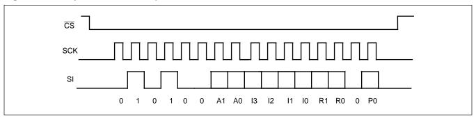
Figure 5. Three-Byte Instruction Sequence (Write)
