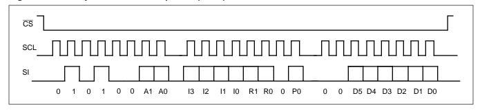
Figure 6. Three-Byte Instruction Sequence (Read)
