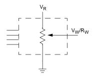
Three terminal Potentiometer; Variable voltage divider
