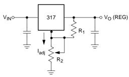
$V_O (REG) = 1.25V (1+R_2/R_1)+I_{adj} R_2$
