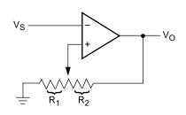
$V_{UL} = \{R_1/(R_1+R_2)\} V_O(max)$  $V_{LL} = \{R_1/(R_1+R_2)\} V_O(min)$
