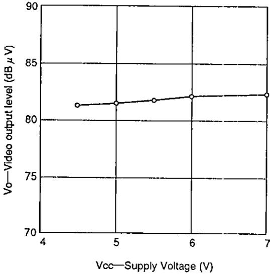
Supply voltage vs. Video modulation depth
