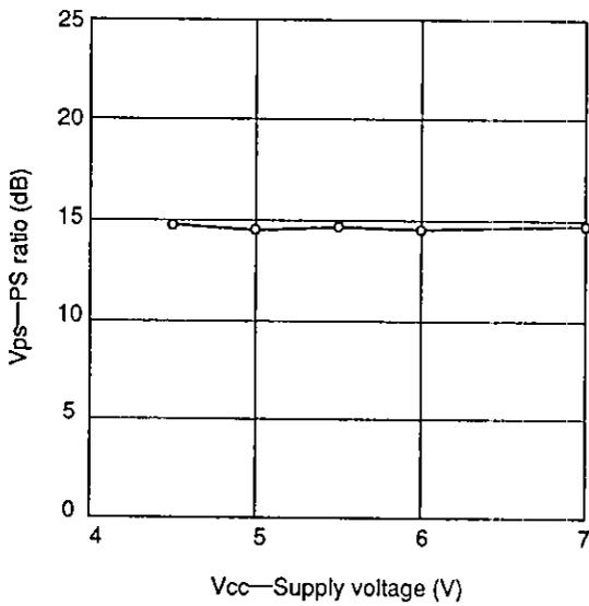
Supply voltage vs. Audio FM modulation sensitivity
