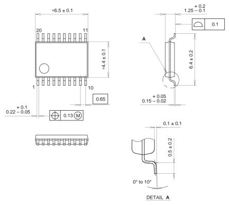
NOTE: Dimension " $\ast$ " does not include mold protrusion.
