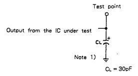
3-state Output Test Load Circuit
