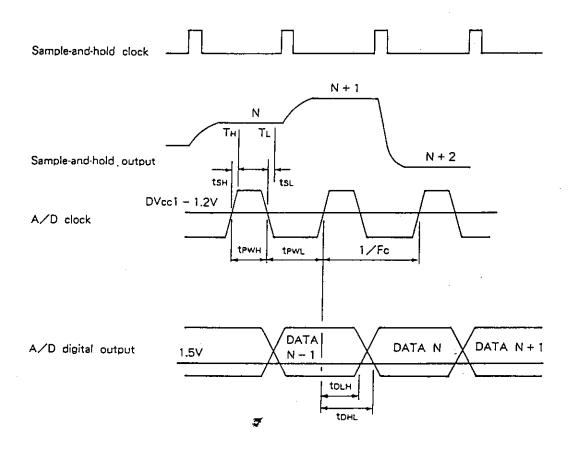
Th is the timing of latching result for the comparator of Vin and Vree in the upper comparators. This the timing of latching result for the comparator of Vin and Vree in the lower comparators.
