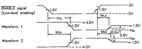
Output waveform of 3-state enable and disable time \*. (\* Enable time=tpzL/tpzH, disable time=tptz/tpHz)
