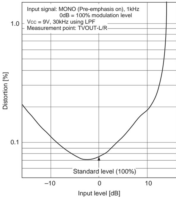
**Input level vs. Distortion characteristics 2 (Stereo)**
