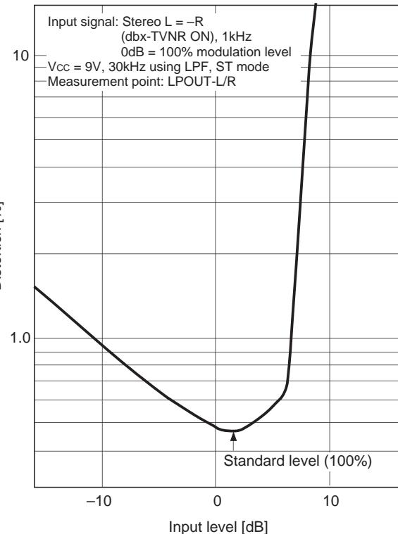
**Input level vs. Distortion characteristics 3 (SAP)**
