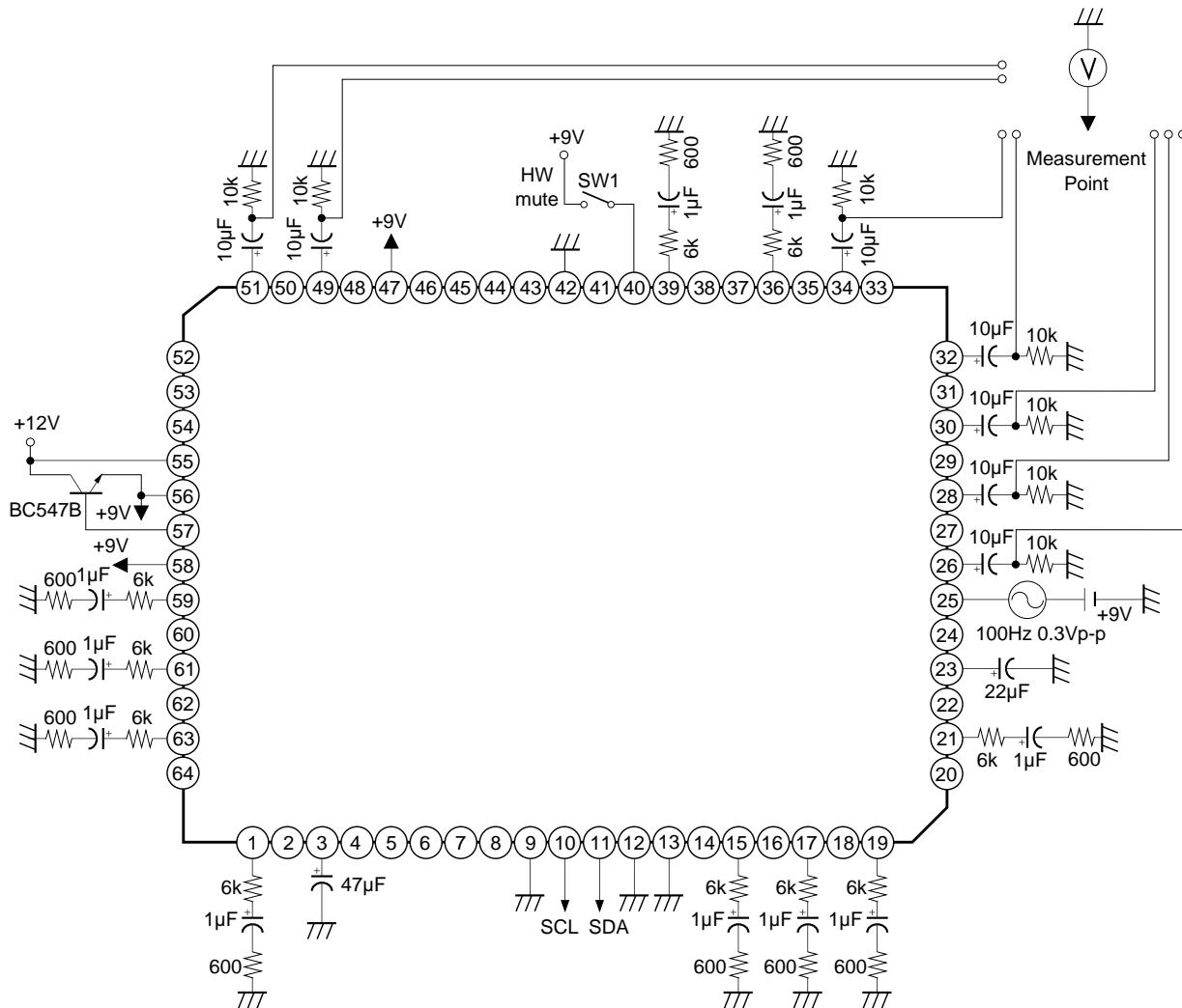
**Fig. 8. Audio system (Ripple Rejection)**
