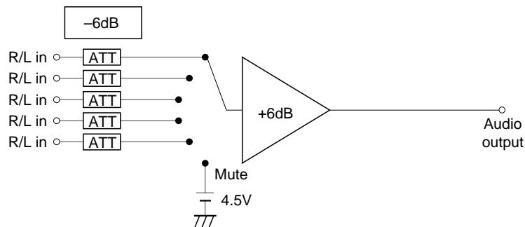
Fig. 2-3. VCR and AUX audio configuration
