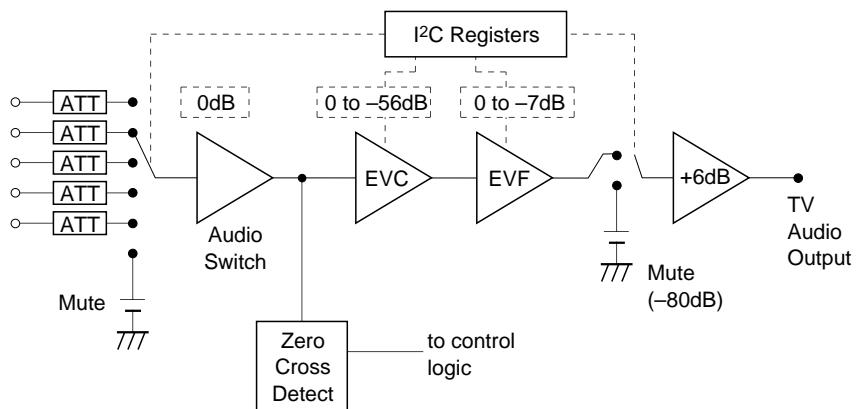
Fig. 2-4. T.V. audio section and Electronic Volume Control
