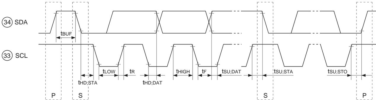
**Fig. 6. I<sup>2</sup>C BUS Control Signal Timing Chart**
