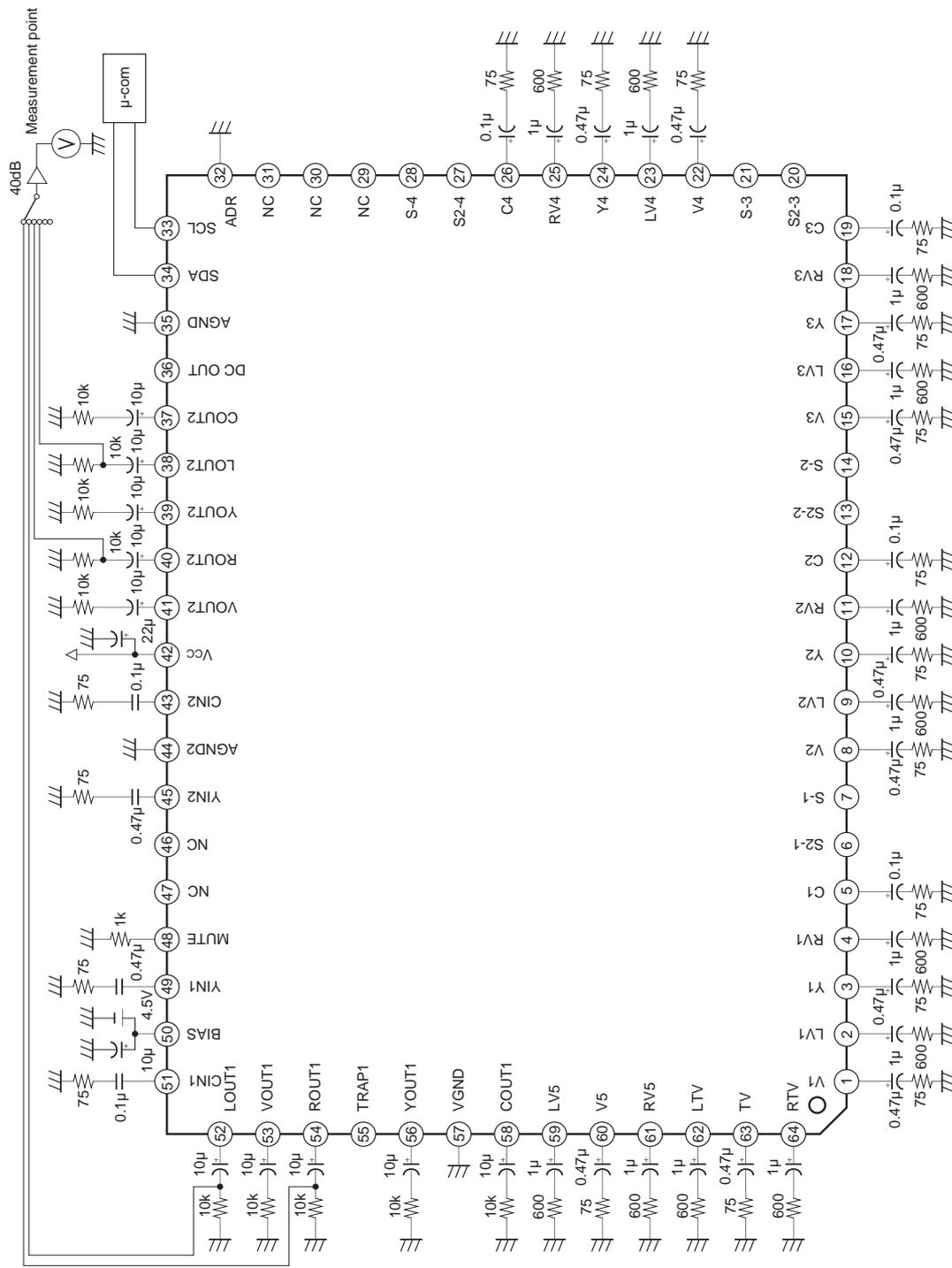
Fig. 5. Audio system (residual noise) measurement circuit
