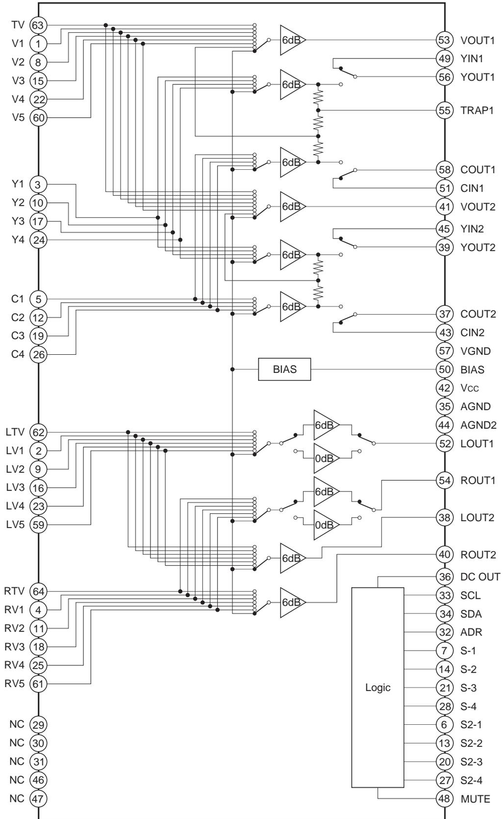
Audio system is attenuated by 6dB for 6kΩ resistor input, and a total gain is 0dB (LOUT1 and ROUT1 can be changed to -6dB).
