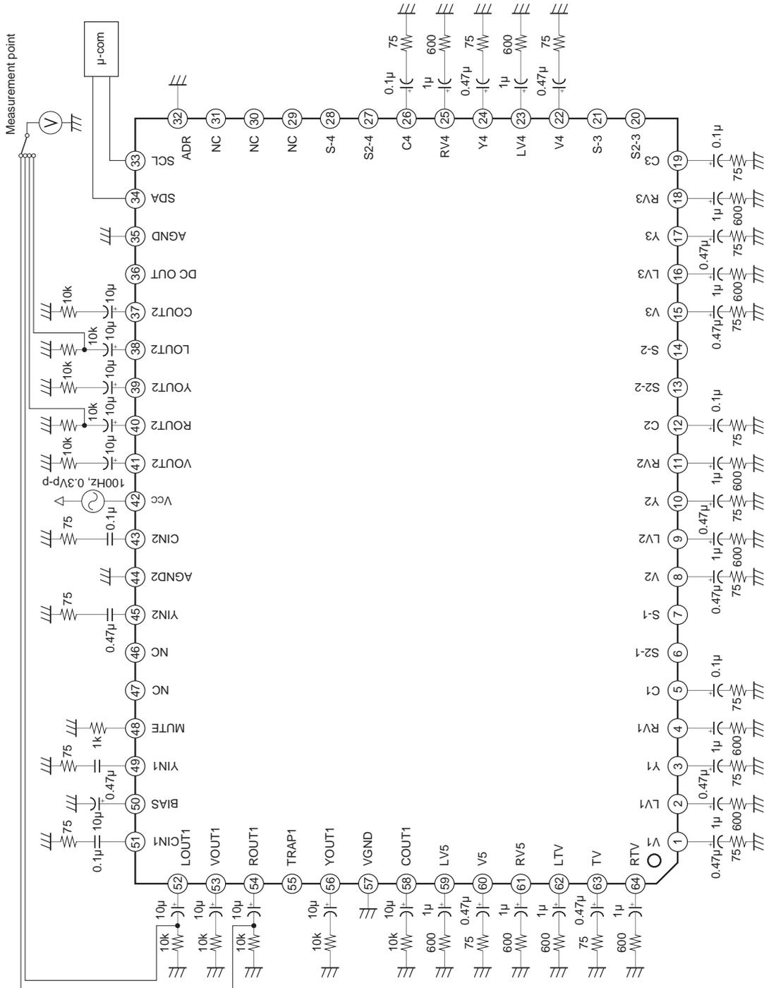
A f=100Hz, 0.3Vp-p signal is applied to Vcc and the output signals from Pins 38, 40, 52 and 54 are measured.
