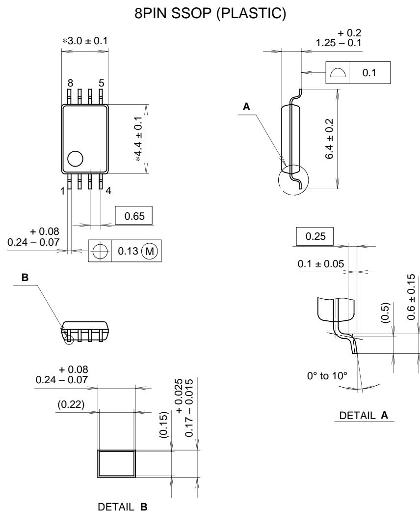
NOTE: Dimension "\*" does not include mold protrusion.
