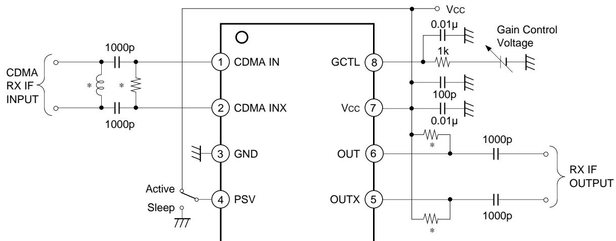
\* Must be adjusting values to result a best impedance matching between BPF filter and this IC.
