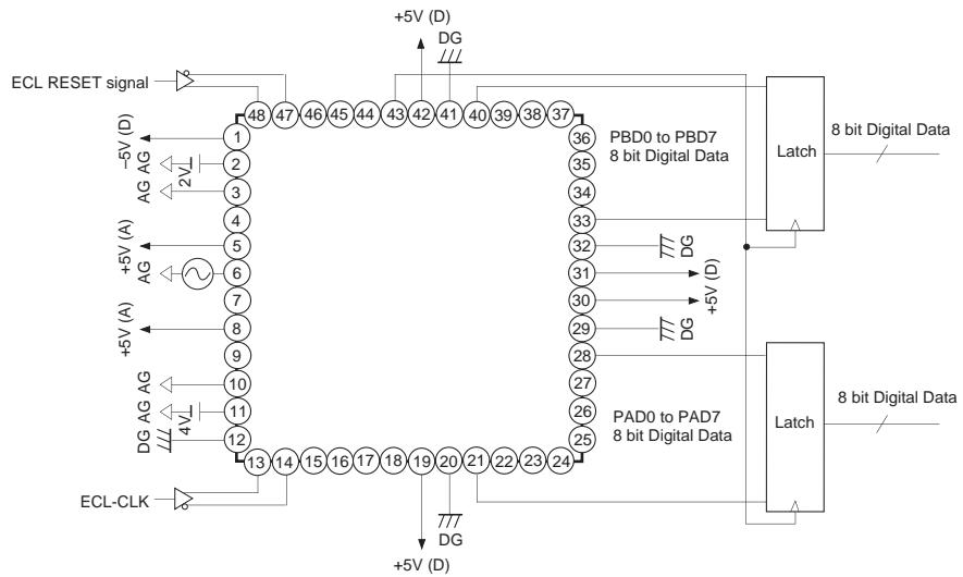
**(2) DMUX PECL input**
