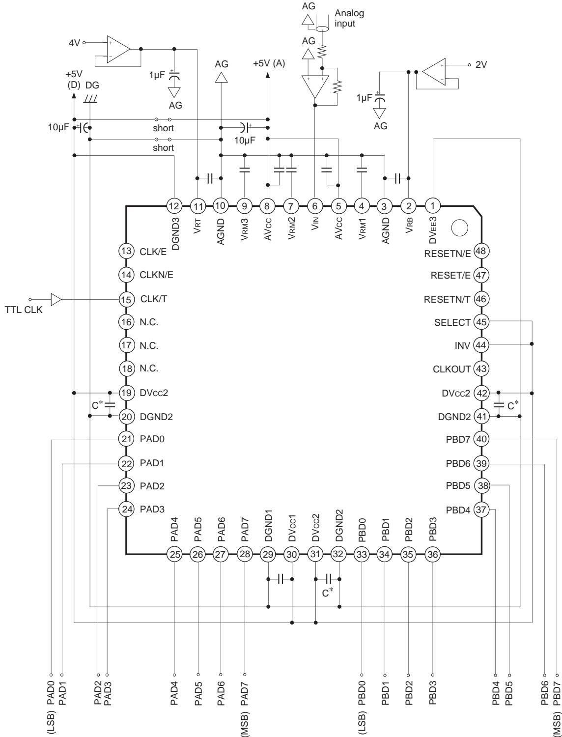
—○— Short the analog system and digital system at one point immediately under the A/D converter. See the Notes on Operation.
