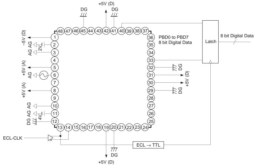
**(5) Straight PECL input**
