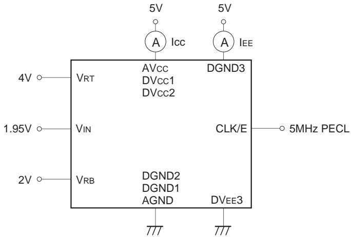
**Integral Linearity Error Measurement Circuit**
