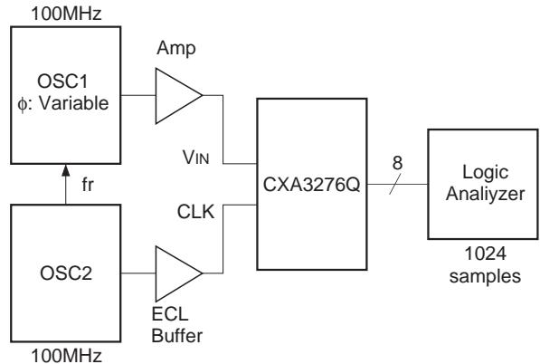
**Aperture Jitter Measurement Method**
