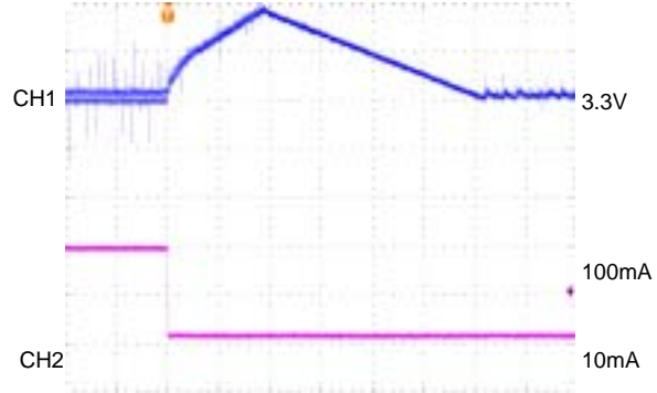
200μsec/div CH1:Vout1, 2, AC-COUPLED, 50mV/div CH2:Iout1, 2, 50mA/div
