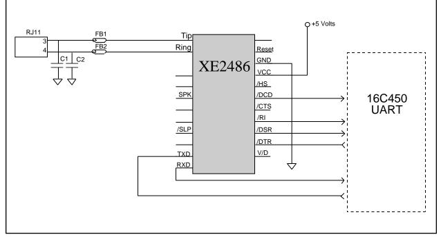
Note: RJ11 Pin assignments reference a 6-pin connector. Tip and Ring are the center pins of all RJ11 jacks.
